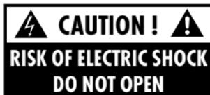
*The lightning flash with arrowhead symbol, within an equilateral triangle, is intended to alert the user to the presence of uninsulated "dangerous voltage" within the unit's enclosure that may be of sufficient magnitude to constitute a risk of electric shock.*
